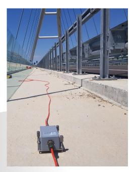
The Digital Array solution can be assembled in various ways to meet the different requirements and applications of field work. The pictures show three different setups. One of the most challenging applications was the coaxial deployment of 6 triaxial units in a 285-meter borehole to monitor microseismic activity in a gas storage plant.
