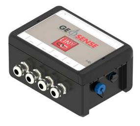
The GeoLogger Linx™ is a range of low-cost battery-powered data loggers for stand-alone monitoring which can be used with all types of vibrating wire sensors such as piezometers, load cells, crack meters, joint meters, strain gauges, pressure cells, weir monitors and extensometers, together with their associated thermistors.
