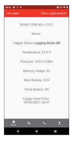
App automatically opens and loads logger configuration when connected.
