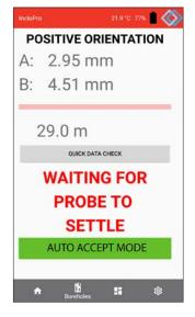
Auto mode provides handsfree automated data recording which ensures consistency & quality of surveys.
