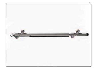
The Geosense Horizontal Portable Inclinometer system is used to measure settlement and/or heave within a horizontal borehole under structures such as embankments, dams, roadways, storage tanks and lanfills.
