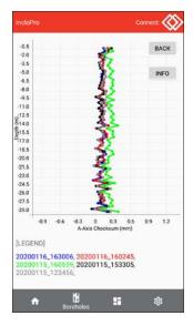
Checksum, cumulative displacement, incremental displacement, mean deviation & absolute position graphs can all be viewed.
