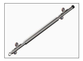
The Geosense Inclined Portable Inclinometer system is used to measure lateral movements and deformations of soil, rock and reatining structures within or on an inclined borehole or surface. Typical applications include monitoring the downstream face of concrete faced rock-filled dams.
