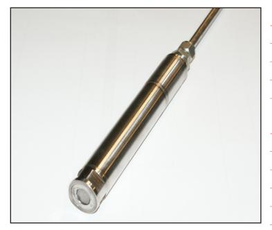
The VWPHT-3600 series High Temperature Piezometers are suitable for the extreme environments of temperature and pressure found within applications such as geothermal heat and enhanced oil recovery systems including steam assisted gravity drainage (SAGD) and cyclic steam stimulation (CSS). They are capable of monitoring high temperatures up to 250°C and pressures up to 34.5 MPa.
