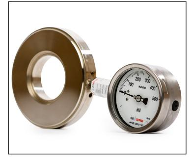
The Geosense® HLC-6000 series Hydraulic Anchor Load Cells consist of a sensitive pressure pad formed by joining two stiff steel discs at their periphery. The void inside the cell is filled with de-aired fluid. When load is applied to the cell the pressure of the inside liquid changes. The changes in pressure correspond directly to the load applied.
