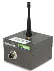
The GeoWAN PT100 RTD Sensor Node allows precision temperature sensing in many different situations. It uses the integrated long range radio transceiver to report its measurements through Senceive's GeoWAN wireless communications network to a GeoWAN Gateway.
