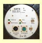
SSBH sensor is a geophysical device designed to measure vibrations in boreholes for DownHole, UpHole and CrossHole surveys.
