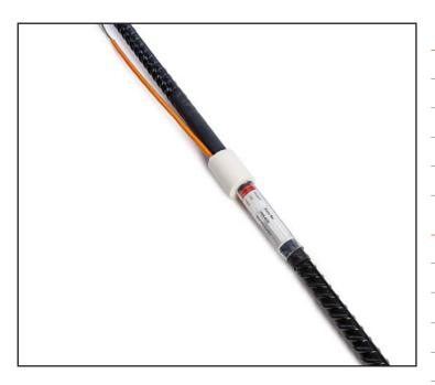
Geosense® VWS-4000 series vibrating wire Sister Bars and Rebar Strain Meters are designed to be embedded in concrete to measure strains due to imposed loads.
