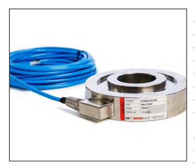
The Geosense® SGLC 7000 series load cell consists of a cylinder of high strength steel with a series of electrical resistance strain gauges connected around the periphery as a Wheatstone Bridge that compensates for unevenly distributed loads and provides a single mV/V signal output.
