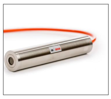
The Geosense® SGP-3400 Series of strain gauge piezometers are designed for monitoring soil pore pressure or changes in water level and are also suitable for dynamic monitoring such as pumping tests.
