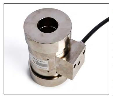
Geosense® VWLC 5000 series Vibrating Wire Anchor Load Cells consist of a cylinder of high strength steel with 3 or 5 vibrating wire strain sensors (depending on capacity) mounted parallel to the longitudinal axis arranged equidistant around the circumference which measure the compression of the cylinder under load.
