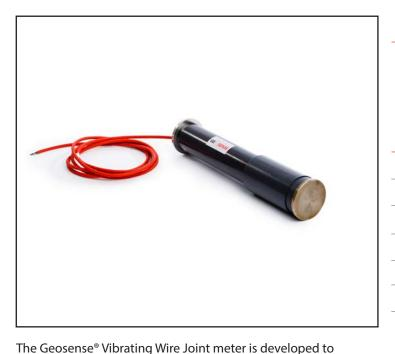
The instrument consists of two parts, a socket and the main body with a waterproof vibrating wire sensing gauge. During construction of the structure, the socket is secured to the form and embedded into a lift of the block to be constructed. After removal of the form, and prior to concreting of adjacent block, the gauge is screwed into the socket, set at the desired range and then embedded into concrete.
