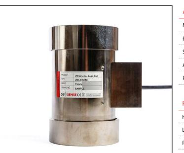
The Geosense® VWLC 5050 series of Vibrating Wire Load Cells consist of a solid cylinder of high strength steel with 3 or 5 vibrating wire strain sensors mounted parallel to the longitudinal axis arranged equidistant around the circumference which measure the compression of the cylinder under load.
