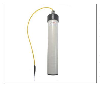
The Geosense® VWM-2000 vibrating wire precision water level monitor utilises a vented vibrating wire force transducer in combination with a cylindrical weight suspended from it to monitor water levels.
