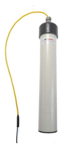
The Geosense® VWM-2000 vibrating wire precision water level monitor utilises a vented vibrating wire force transducer in combination with a cylindrical weight suspended from it to monitor water levels.
