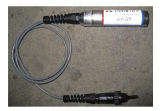
YieldPoint's *d-PIEZO* provides reliable and repeatable readings of pressure in a wide range of conditions. The technology employed allows utilization in harsh conditions such as brackish, hot and acid water often met in mines.
