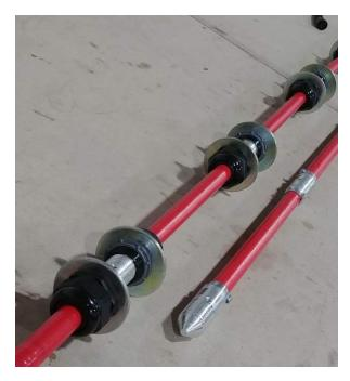
The high-profile anchor allows an excellent transfer of force from the surrounding ground through a bentonite cement grout. A 75mm borehole is adequate.
