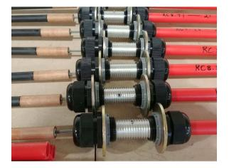
Delivered fully integrated, the extensometer comes coiled on a 120cm diameter, fully ready for installation and grouting. No calibration is required and manual tightness adjustment of the anchors is possible.
