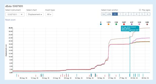
This software features a very powerful zooming capability that allows engineers to analyze the effect of individual blasts or seismic events. By establishing relationships between the magnitude and distance (concept of scaled distance) of events and the corresponding "micro-damage" to the walls of excavations, powerful predictive models can be developed.
