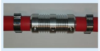
YieldPoint MPBX extensometers are also available for use in soil (road settlement) or in trenches (slopes).
