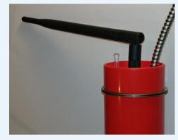
Clusters of up to 16 instruments can be monitored and networked via YieldPoint's **wired Ethernet Gateways** or a 900MHz low cost Zigbee wireless mesh solution. These solutions interface with TCP/IP or WiFi networks.
