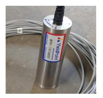
**d-Tilt** and **BluTilt** are full 360 arcdeg triaxial tiltmeters for very precise measurement (0.001 arcdeg resolution) of changes in inclination. These instruments use a very low noise MEMS accelerometer that enables a resolution of 0.001 arcdeg with a 24hr stability of +/-0.001 arcdeg.
